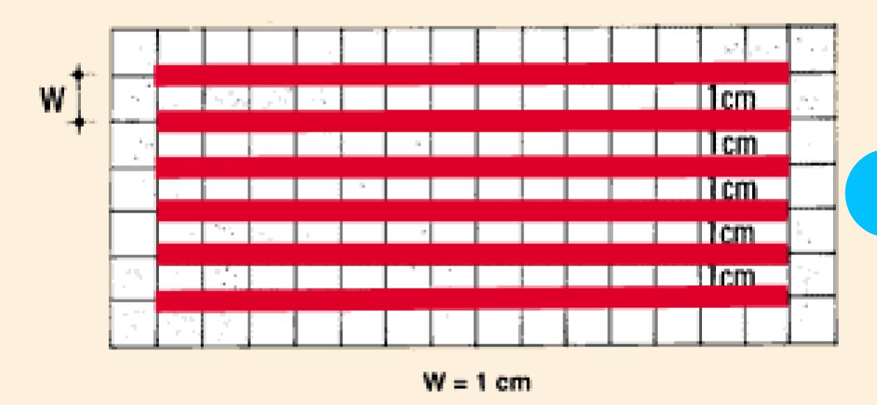
3. Place the sheet of transparent paper over the plan or map of the area you need to measure, and attach it securely with drawing pins or transparent tape. 2. On this paper, draw a series of strips, by drawing a series of parallel lines at a regular, fixed interval. Choose this strip width W to represent a certain number of metres.
