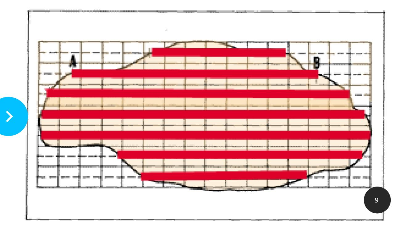
6. Multiply this sum of real distances (in metres) by the equivalent width of the strip W (in metres) to obtain a rough estimate of the total area in square metres.
