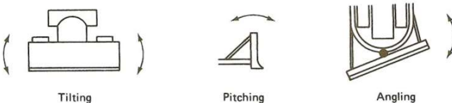
FIGURE 4-8: Dozer blade adjustments.
