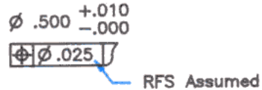
HOLE SPECIFICATION AND POSITION TOLERANCE
