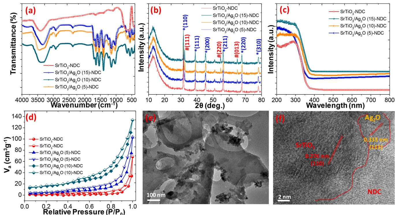
Fig. 1. (a) FTIR spectra (b) XRD spectra (c) DRS Spectra (e) N<sub>2</sub> adsorption desorption isotherm (e) TEM and (f) HRTEM of SrTiO<sub>3</sub>/Ag<sub>2</sub>O-NDC based nanocomposites.
