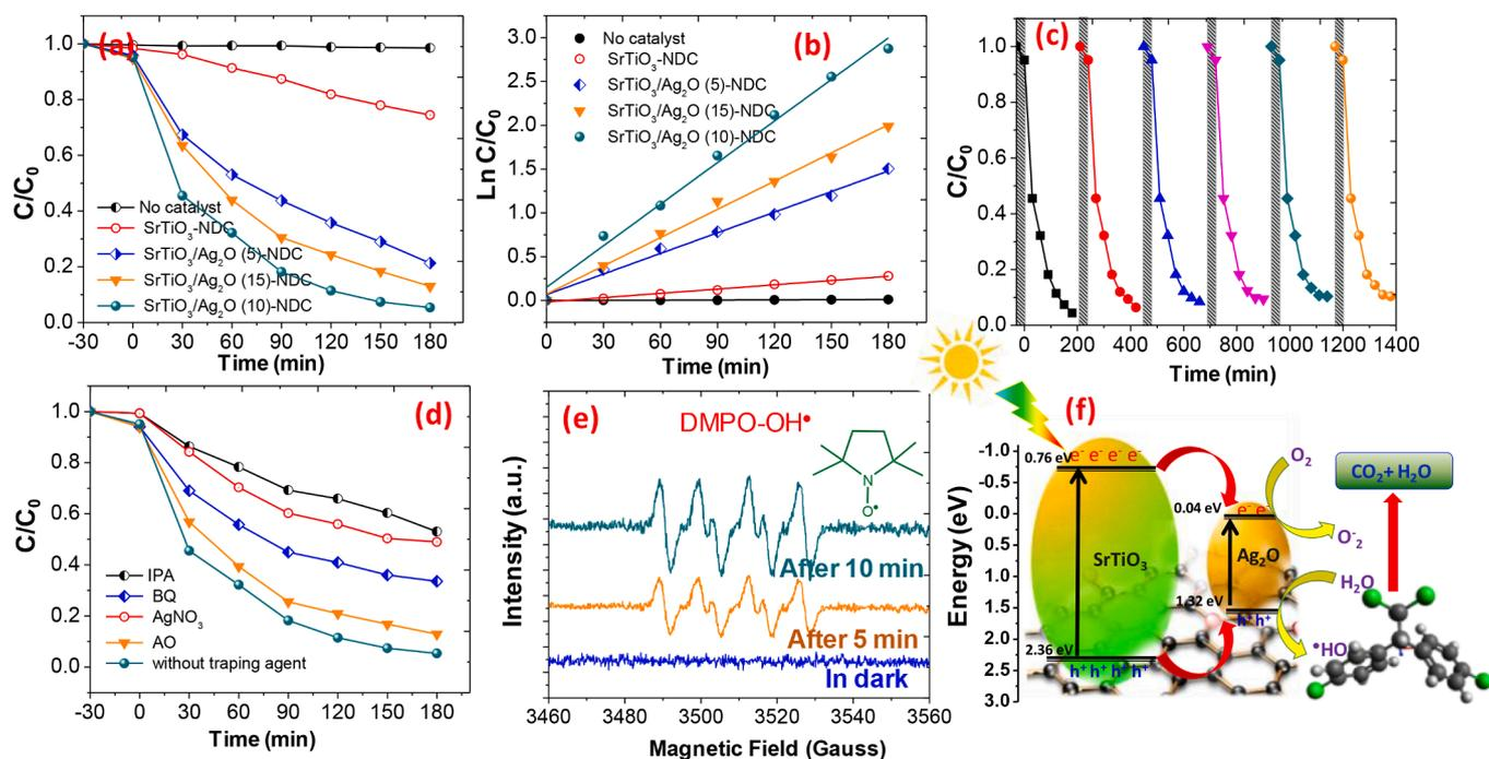
Fig. 3. (a) Effect of catalysts (b) photodegradation kinetics (c) reusability (d) effect of trapping agents (e) ESR spectral and (f) schematic band structure and charge-transfer process during the degradation of DDT.
