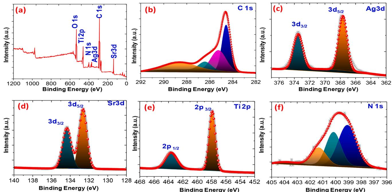
Fig. 2. (a) Wide XPS (b) C1s(c) Ag3d(e) Sr3d(e) Ti2p and (f) N1s of SrTiO<sub>3</sub>/Ag<sub>2</sub>O(10)-NDC nanocomposites.
