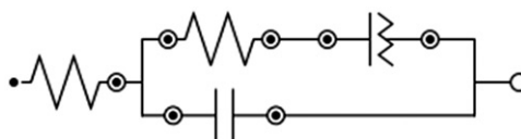
Figure 7. Equivalent circuit to fit the experimental data of PUIEtA-2.
