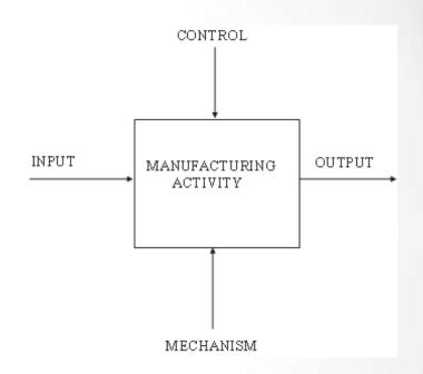
The specific activity, inputs, outputs, mechanisms, and controls are defined by the situation being modeled
