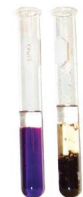
Hexane does not react with purple \text{KMnO}_4 (left); cyclohexene (right) reacts, producing a brown-black precipitate of \text{MnO}_2 .
