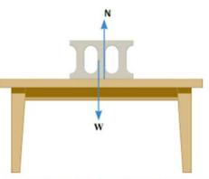
The normal force N is one component of the force that a surface exerts on an object with which it is in contact, namely, the component that is perpendicular to the surface.
