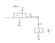
A 5.00-kg object placed on a frictionless, horizontal table is connected to a string that passes over a pulley and then is fastened to a hanging 9.00-kg object, as in Figure P5.24. Draw free-body diagrams of both objects. Find the acceleration of the two objects and the tension in the string.
