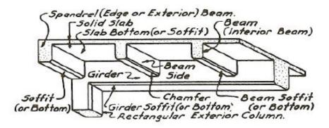
a. Slab-beam-and-girder floor
