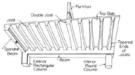
b. Concrete joist floor
