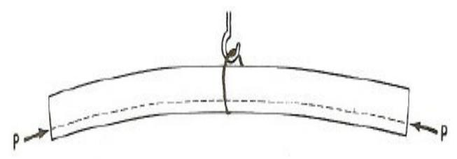
**FIGURE 12-11**: Lifting prestressed beam at the center.
