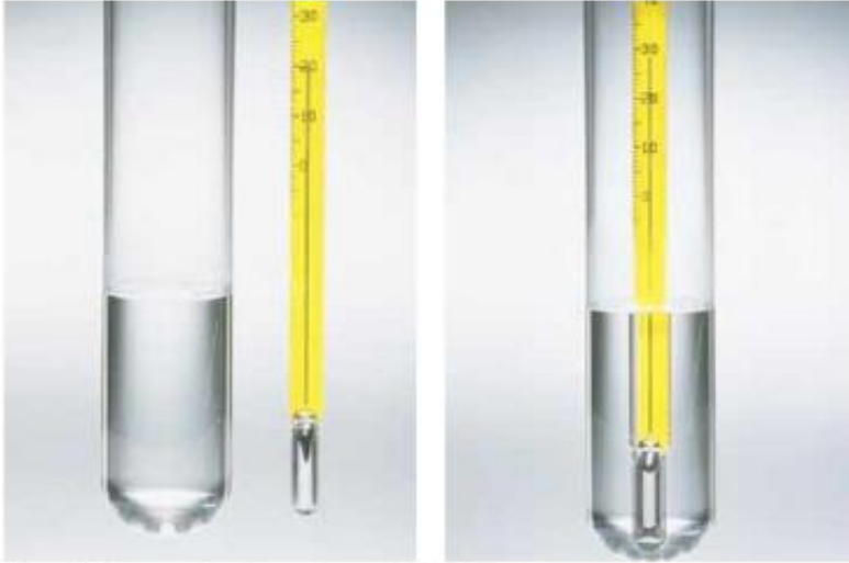
Figure 19.2 As a result of thermal expansion, the level of the mercury in the thermometer rises as the mercury is heated by water in the test tube.
