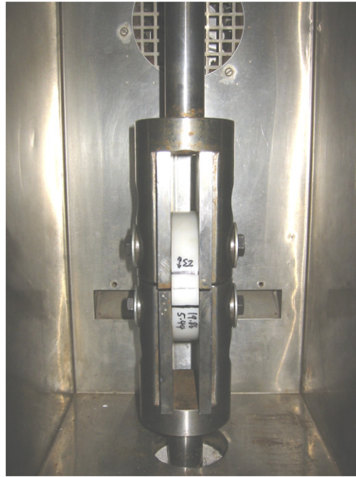
Fig. 3. Assembly of the test rig.
