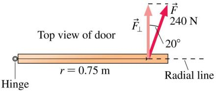
**PREPARE** In the figure, the radial line is shown drawn from the pivot—the hinge—through the point at which the force  $\vec{F}$  is applied. We see that the component of  $\vec{F}$  that is perpendicular to the radial line is  $F_{\perp} = F \cos 20^{\circ} = 226$  N. The distance from the hinge to the point at which the force is applied is r = 0.75 m.
