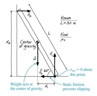
**PREPARE** The ladder is a rigid rod of length *L*. To not slip, both the net force and net torque on the ladder must be zero. The figure shows the ladder and the on it.
