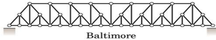
Commonly Used Bridge Trusses
