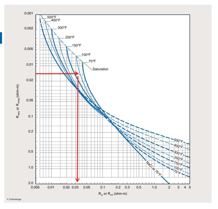
These charts convert equivalent water resistivity,  $R_{weq}$ , from Chart SP-1 to actual water resistivity,  $R_w$ . They may also be used to convert  $R_{mf}$  to  $R_{mfeq}$  in saline muds.
