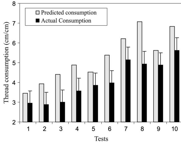
The weakness of the theoretical models can be explained by the negligence of many other parameters such as the yarn tension, the cloth compression and the stitch distortion.
