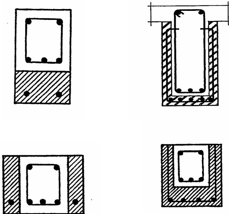
Fig. 4 Additional reinforcements for beams
