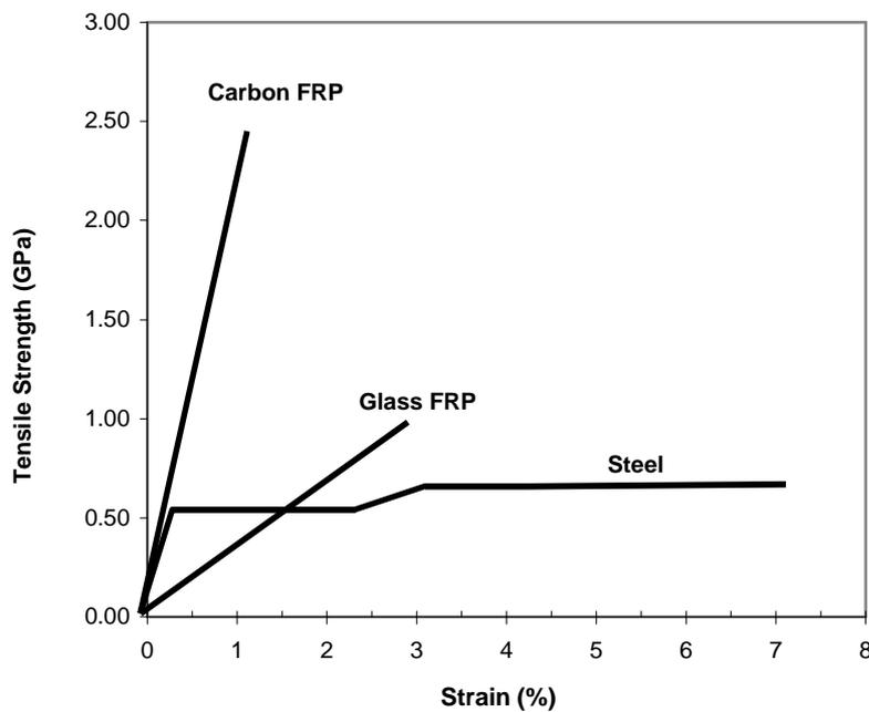
Fig. 6 Typical stress-strain relationships of FRP composites and mild steel
