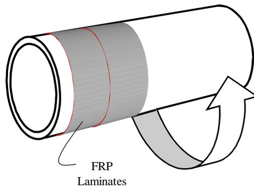
Fig. 10 Rehabilitation of pipes with FRP composites
