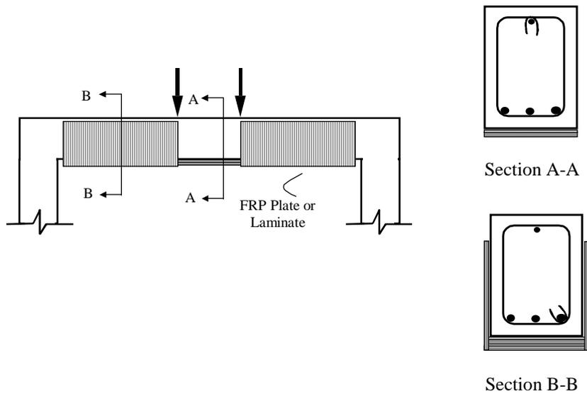
(b) Flexural and shear strengthening
