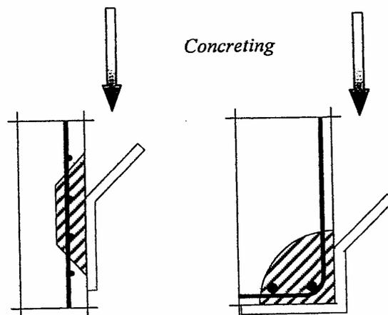
Fig. 1 Patch repairs to damaged concrete surfaces
