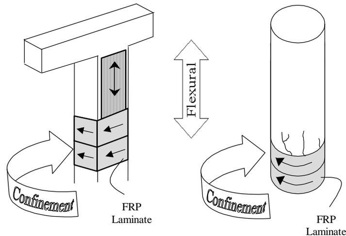
Fig. 8 Rehabilitation of columns with FRP composites
