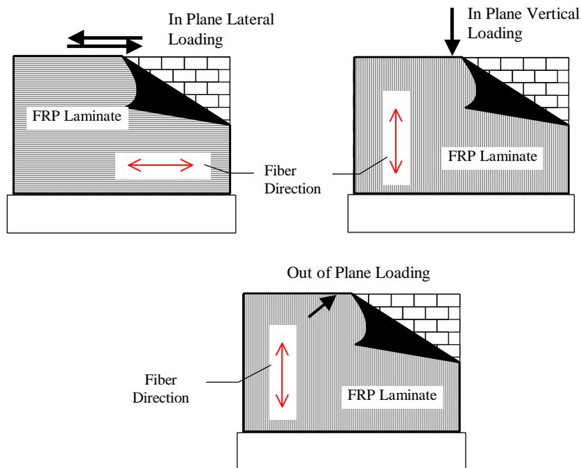
Fig. 9 Rehabilitation of walls with FRP composites
