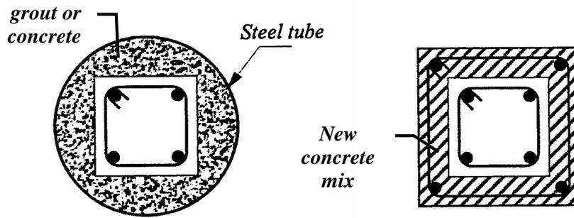
Fig. 3 Increasing cross-sections of columns
