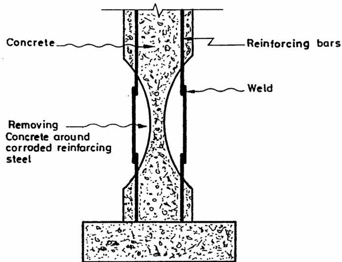
Fig. 2 Replacement of corroded reinforcement
