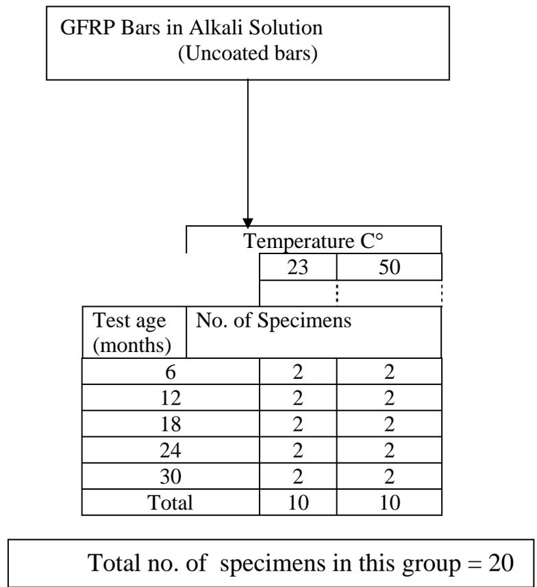
Figure 3: Experimental program for GFP bars immersed in alkali solution
