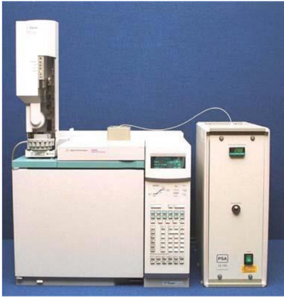
Schematic diagram and photograph of the GC-AFS system.
