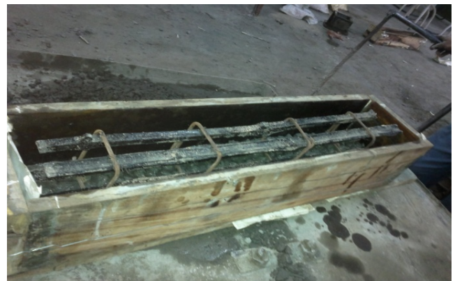
Fig.7 Concrete and bamboo stick in the mould
