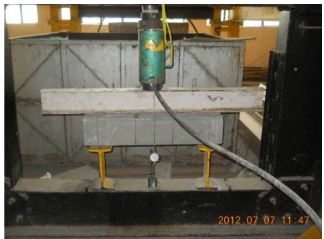
Fig.8 Setup for testing of bamboo reinforced beam in pure bending
