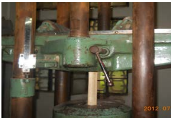
Fig. 4 Bamboo stick under tension in universal testing machine
