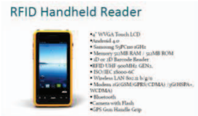
Figure 2: The RFID Handheld Reader and its Characteristics
