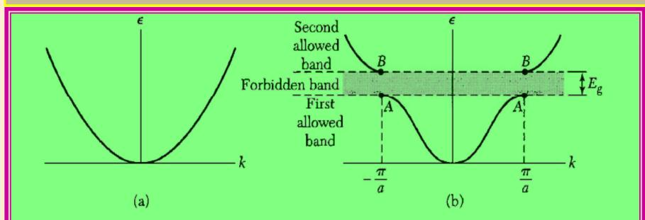
**Figure 2** (a) Plot of energy  $\epsilon$  versus wavevector k for a free electron. (b) Plot of energy versus wavevector for an electron in a monatomic linear lattice of lattice constant a. The energy gap  $E_g$  shown is associated with the first Bragg reflection at  $k = \pm \pi/a$ ; other gaps are found at higher energies at  $\pm n\pi/a$ , for integral values of n.
