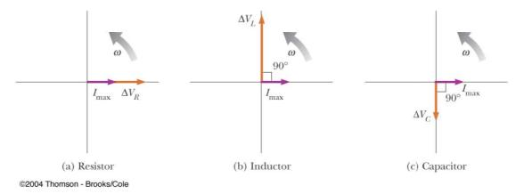
Because the phasors are rotating vectors, the voltage phasors can be combined using vector addition as in the following figure.
