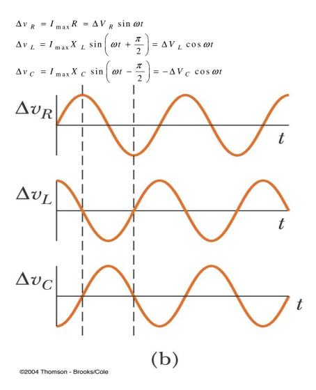
Phase relationships between the voltage and current phasors for (a) a resistor, (b) an indicator, and (c) a capacitor connected in series are shown in following figure.
