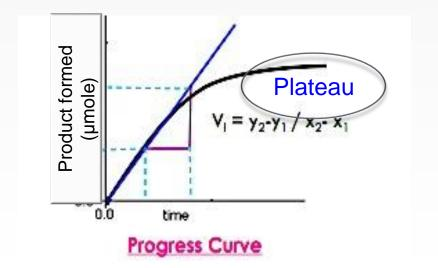
**Progress curve** is a graphic representation of a enzyme-catalyzed reaction in which the product or the substrate conc. is plotted against time
