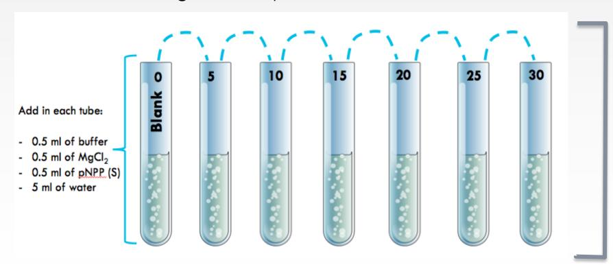
Place in a water bath maintained at 37 °C for 5 minutes
