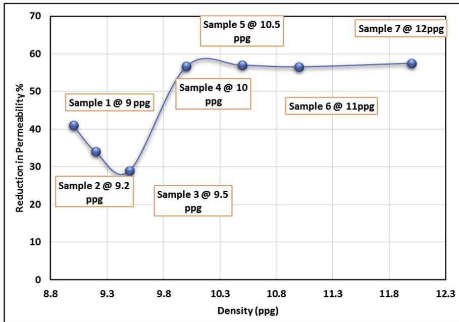
Fig. 12. Effect of the density on reduction in permeability of the ceramic disk.
