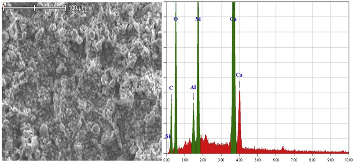
Fig. 15. SEM analysis of  $\text{CaCO}_3$  filter cake.
