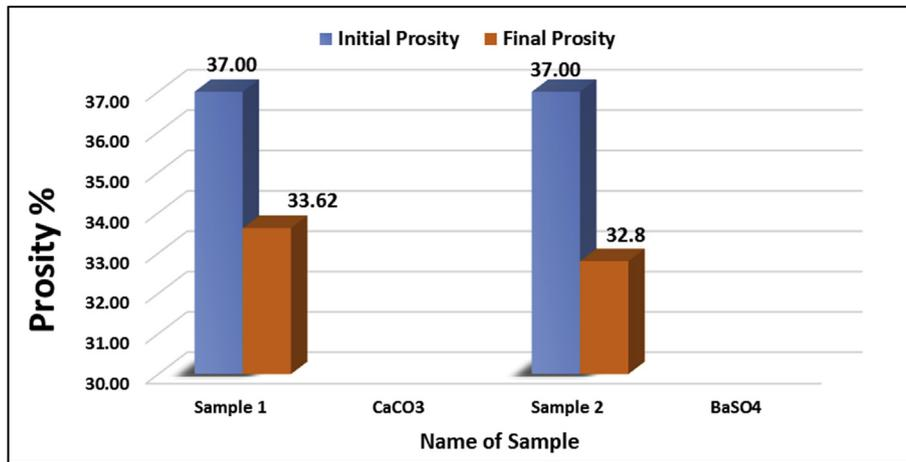
Fig. 11. Effect of the drilling fluids (CaCO<sub>3</sub> and BaSO<sub>4</sub>) on porosity of the ceramic disk.
