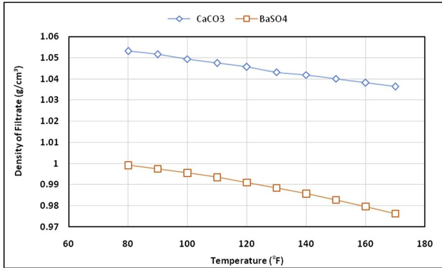
Fig. 4. Change of filtrate fluid density with temperature (samples with different weighting materials).
