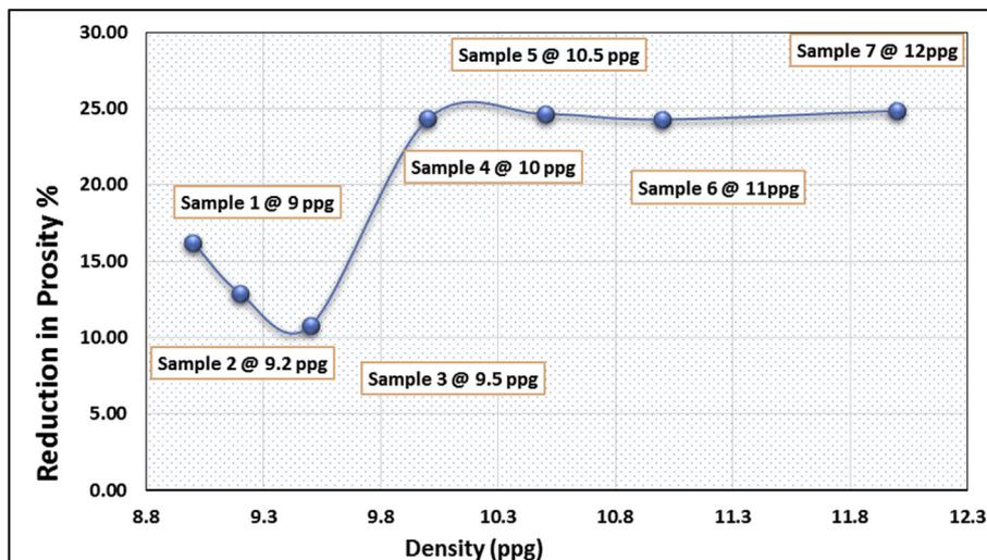
Fig. 10. Density effect on reduction of porosity of the ceramic desk.
