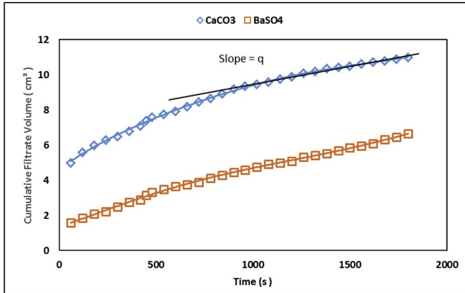
Fig. 9. Cumulative filtrate volume recorded for CaCO<sub>3</sub> and BaSO<sub>4</sub> samples with time (Li et al., 2005).
