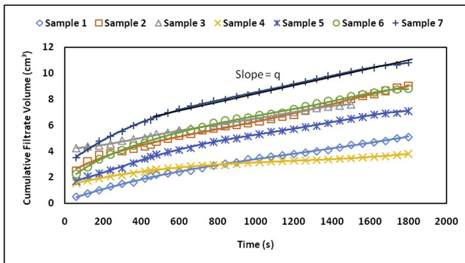
Fig. 8. Cumulative filtrate volume recorded for samples with different densities (Li et al., 2005).
