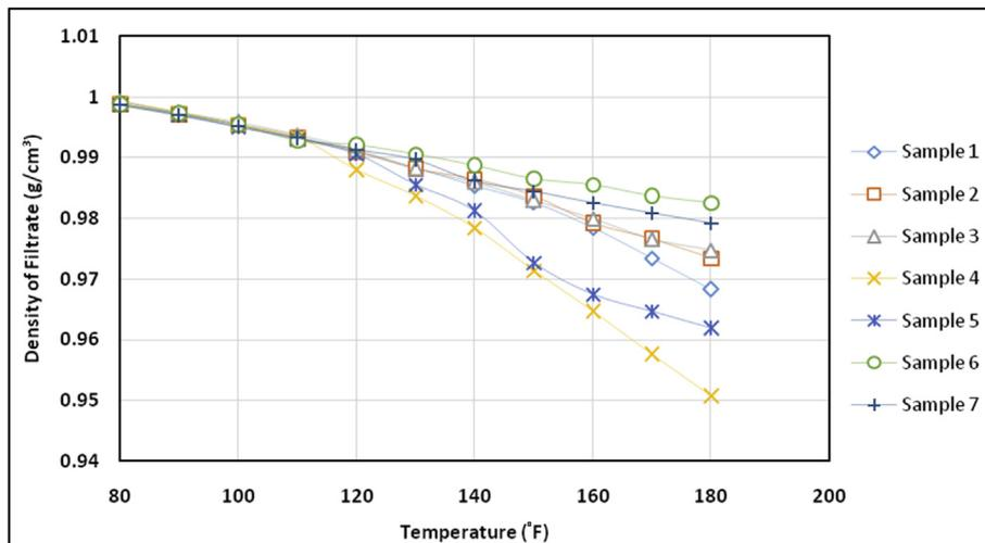
Fig. 3. Change of filtrate fluid density with temperature (Samples with different densities).
