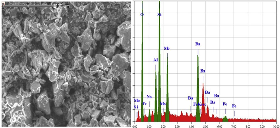
Fig. 14. SEM analysis of filter cake of drilling fluid of density of 9.5 lb/gal (Sample 3).
