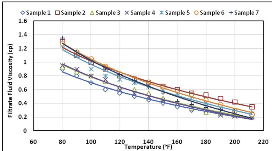
Fig. 5. Change in filtrate viscosity with temperature (Samples with different densities).
