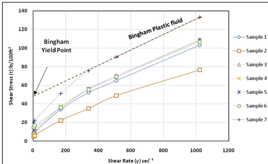
Fig. 1. Shear rate vs. shear stress (samples with different densities).
