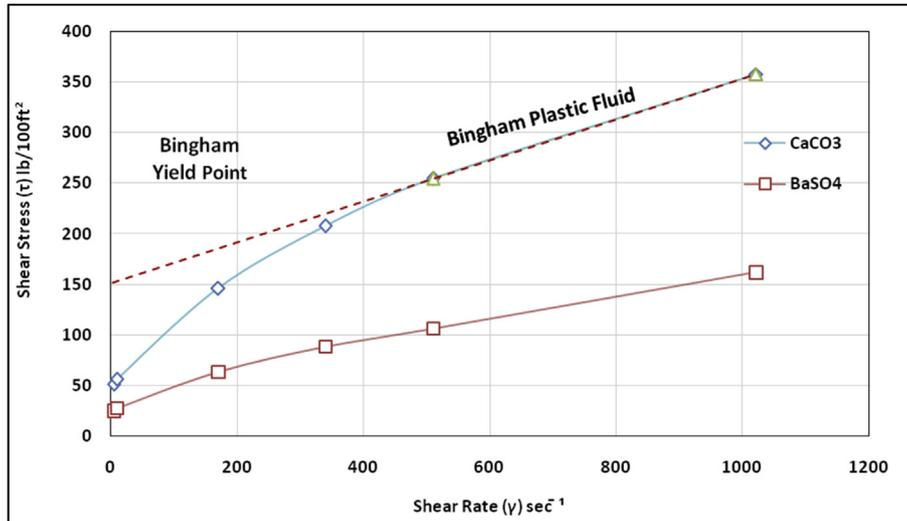
Fig. 2. Shear rate vs. shear stress (samples with different weighting materials).
