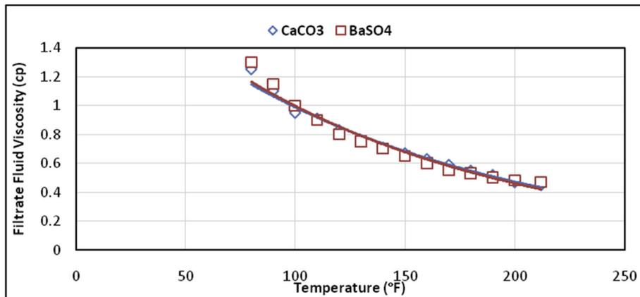
Fig. 6. Change in filtrate viscosity with temperature (CaCO<sub>3</sub> & BaSO<sub>4</sub>).
