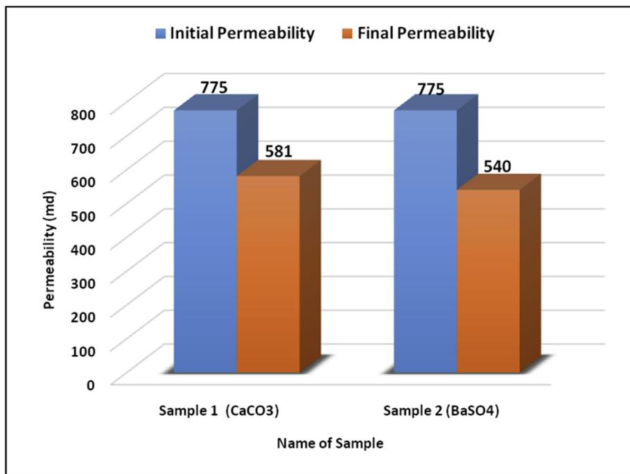
Fig. 13. Effect of the drilling fluids (CaCO<sub>3</sub> and BaSO<sub>4</sub>) on the permeability of the ceramic disk.
