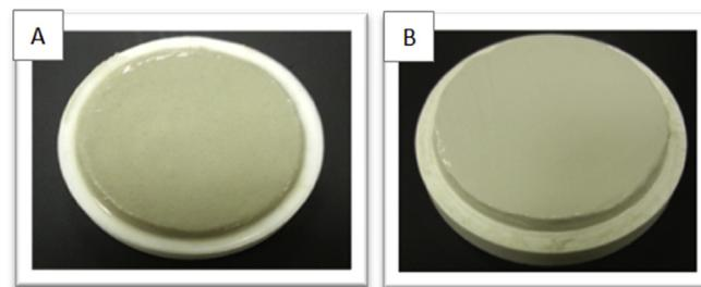
Fig. 7. The filter cake samples obtained from filtration loss tests, a) Samples with different densities (sample3) and b) CaCO<sub>3</sub> weighting fluid (sample1).
