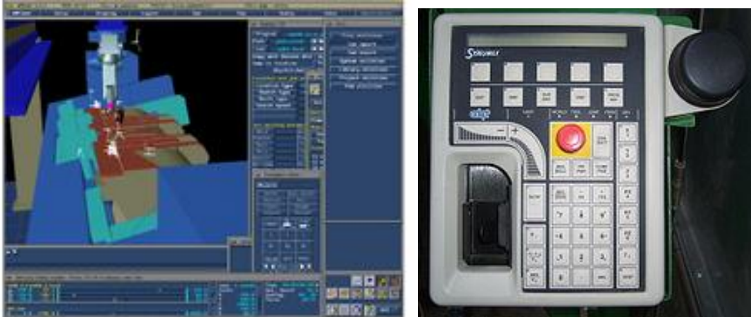
Fig 2.5 Industrial Robot programming and teaching pendant
