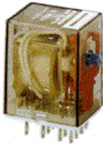
Fig. 3.10 A typical industrial relay.
