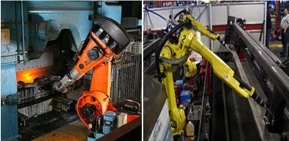
Fig 2.1 Industrial Robot in foundry process(left side) and in welding process in right side.
