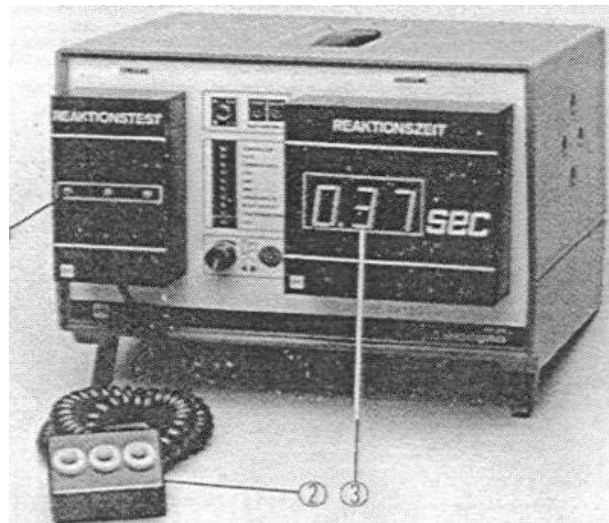
Figure 1.1 Experimental setup for measuring Reaction time
