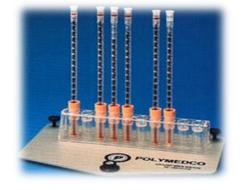
In this technique, anticoagulated whole blood are allowed to sediment under the effect of gravity, using a narrow vertical tube called <u>Westergren's tube</u>.
