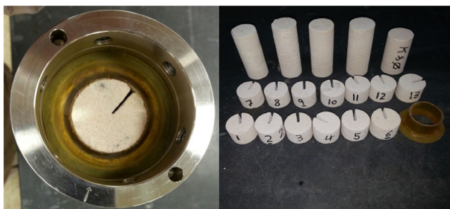
Fig. 2. The developed core holder and the testing cores.
