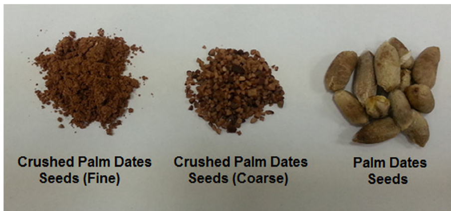
Fig. 4. Date palm seeds before and after crushing and sieving.
