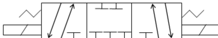
e. Double solenoid & return springs (5/3) valve.
