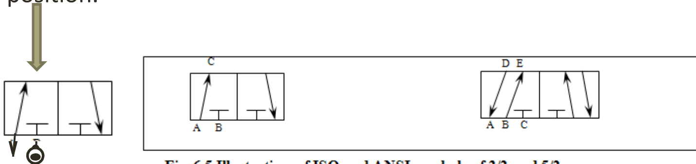
Fig. 6.5 Illustration of ISO and ANSI symbols of 3/2 and 5/2 ways directional valve.
