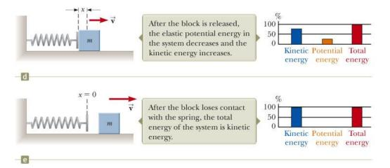
In d, the block has been released and is moving to the right while still in contact with the spring.
