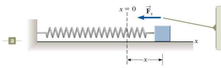
When *x* is positive (stretched spring), the spring force is directed to the left.
