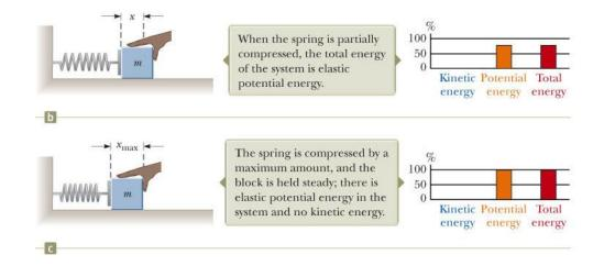
Between b and c, the hand has done work on the system.
