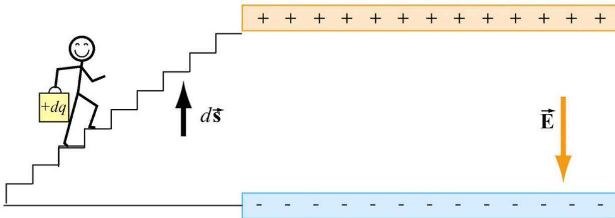
Let the capacitor be initially uncharged. In each plate of the capacitor, there are many negative and positive charges, but the number of negative charges balances the number of positive charges, so that there is no net charge, and therefore no electric field between the plates. We have a magic bucket and a set of stairs from the bottom plate to the top plate.
