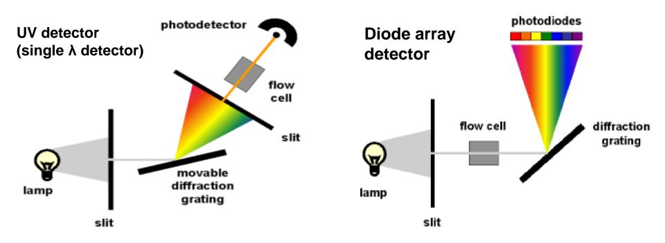
Photodiode array allows for the best wavelength(s) to be selected for actual analysis. This is particularly important when no information is available on molar absorptivities at different wavelengths. The second major advantage is related to the problem of peak purity, absorbance rationing at several wavelengths is particularly helpful in deciding whether the peak represents a single compound or, is in fact, a composite peak.
