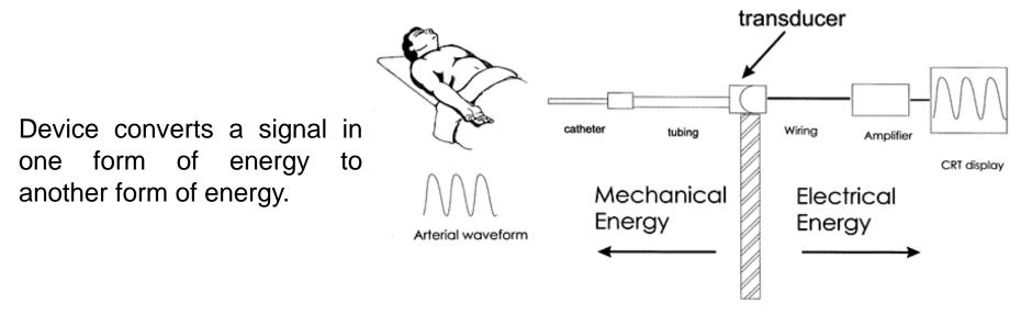
**Transducer:** a device that converts a chemical or physical property, such as pH or photon intensity, to an easily measured electrical signal, such as a voltage or current.
