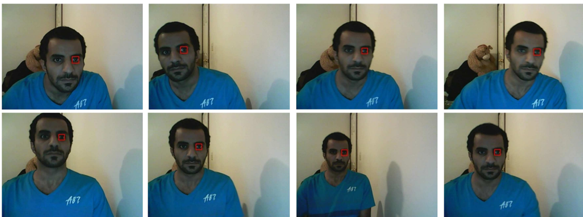
Figure 12: Sequence of frames of tracking a human eye
