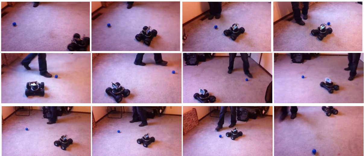
Figure 10: Sequence of frames of tracking a blue ball
