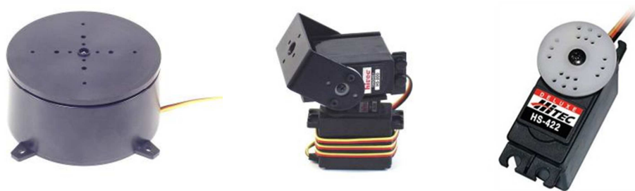
Figure 4: rotating base, pan and tilt kit and the servo motor
