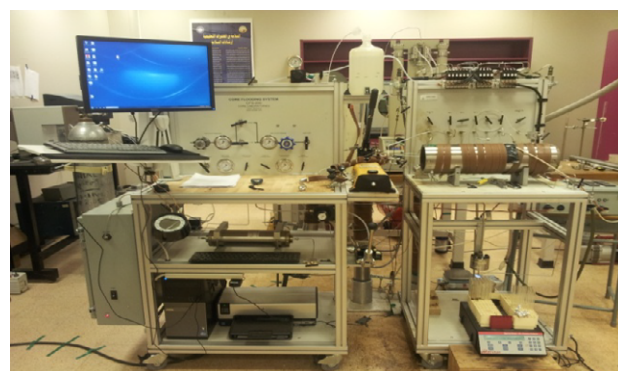
Figure 1: Core flooding system CFS-200.
