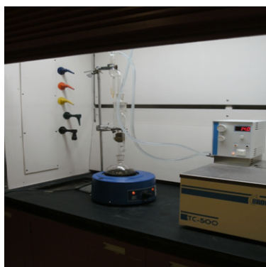
Figure 5: Soxhlet extractor apparatus.
