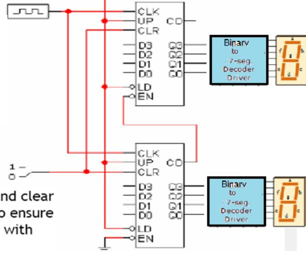
The two four-bit counters share clock and clear inputs. Sharing the clock is important to ensure that the two counters are synchronized with respect to each other.
