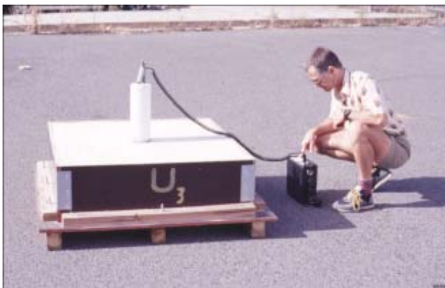
FIG. 4.4. Calibration of a portable spectrometer on a transportable calibration pad.
