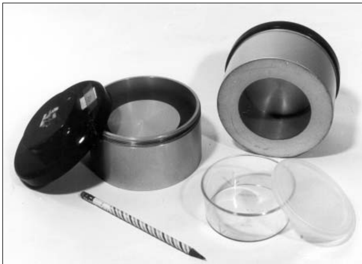
FIG. 4.5. Marinelli type metal and cylindrical plastic containers for laboratory sample analyses.
