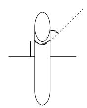
b- mercury  $\theta=130$  ,  $r=1\,mm$  ,  $\gamma=13.6 {{\it KN}\over {\it m2}}$  , surface tension = 0.514
