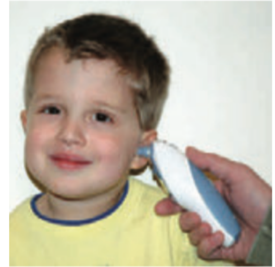
Figure 40.8 An ear thermometer measures a patient's temperature by detecting the intensity of infrared radiation leaving the eardrum.
