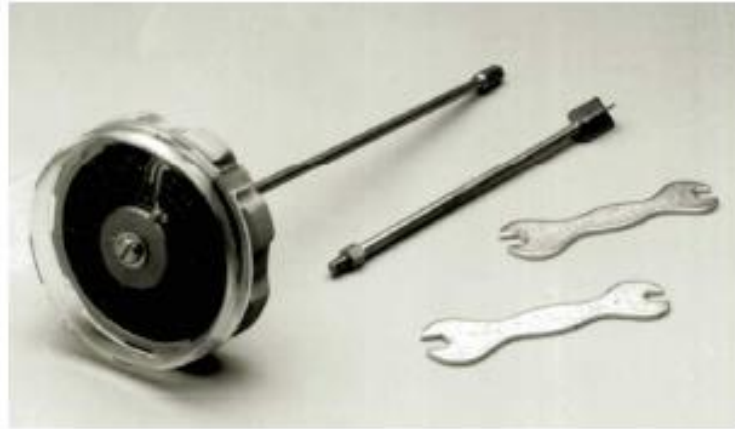
Figure 12.47 Laboratory vane shear test device (Courtesy of ELE International)
