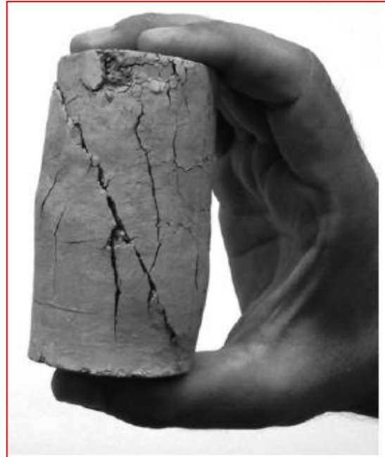
Failure by shear
