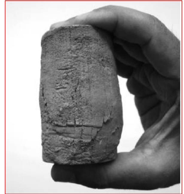
Failure by Bulging
