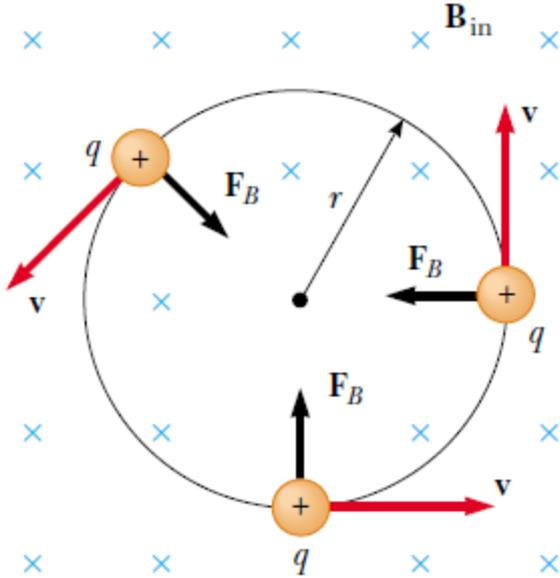
**Active Figure 29.18** When the velocity of a charged particle is perpendicular to a uniform magnetic field, the particle moves in a circular path in a plane perpendicular to  $\mathbf{B}$ . The magnetic force  $\mathbf{F}_B$  acting on the charge is always directed toward the center of the circle.
