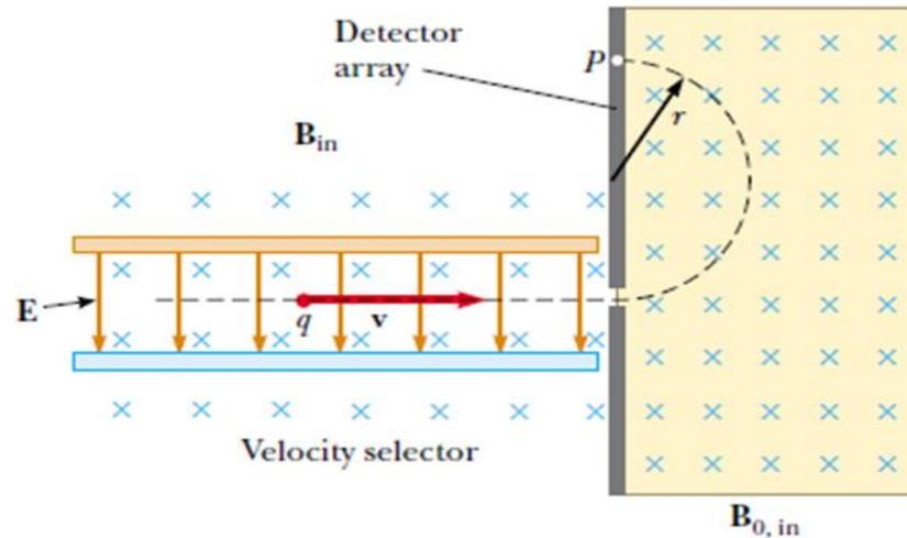
**Active Figure 29.24** A mass spectrometer. Positively charged particles are sent first through a velocity selector and then into a region where the magnetic field  $B_0$  causes the particles to move in a semicircular path and strike a detector array at  $P$ .
