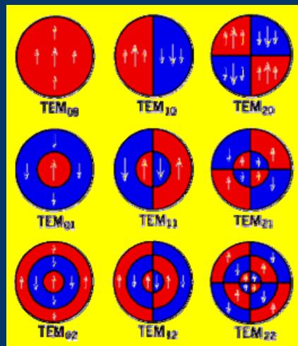
*Electric field distribution of a few of the lowest order resonant modes of a cylindrical cavity.*
