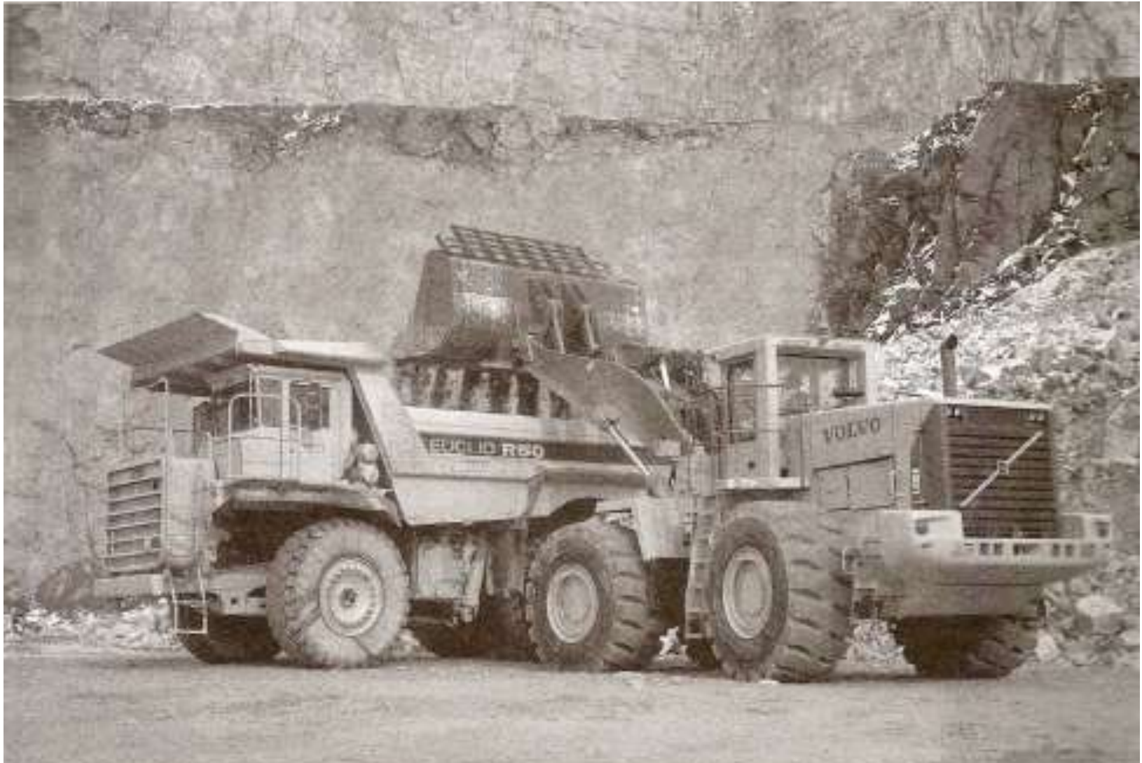
FIGURE 4-26: 41-ton rear-dump truck. (Courtesy of Volvo Construction Equipment North America, Inc.)
