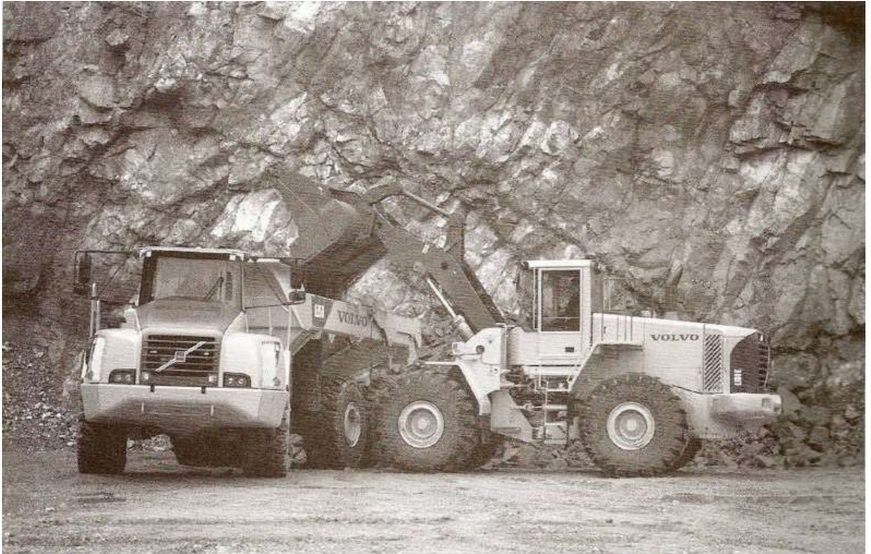
FIGURE4-9: Articulated wheel loader with articulated hauler. (Courtesy of Volvo Construction Equipment North America, Inc.)
