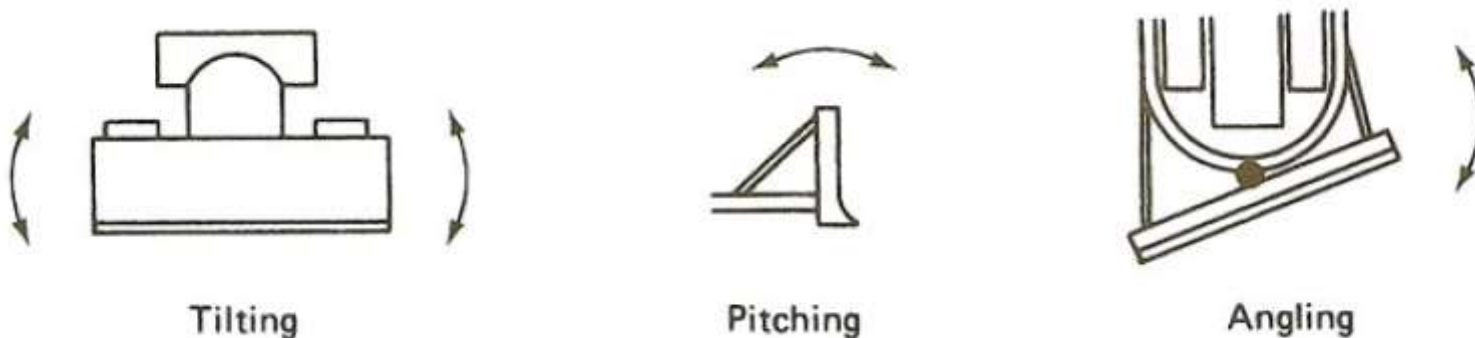
FIGURE 4-8: Dozer blade adjustments.
