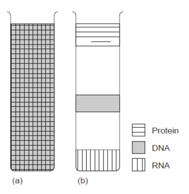
Illustration showing separation by equilibrium-density-gradient centrifugation.
