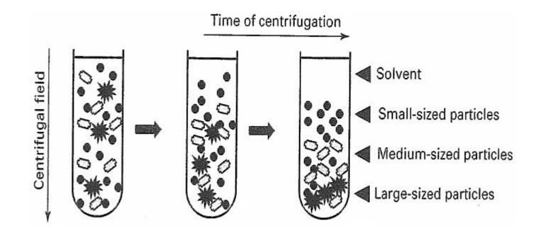
Based on differences in sedimentation rate of the sample particles of different size, shape and density.
