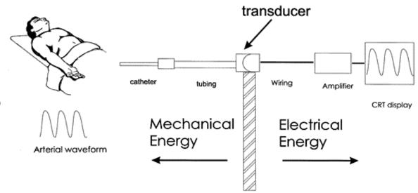
**Transducer:** a device that converts a chemical or physical property, such as pH or photon intensity, to an easily measured electrical signal, such as a voltage or current.
