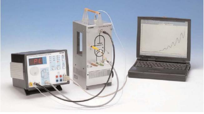
Fig.1: Set-up for the Franck-Hertz experiment with PC.
