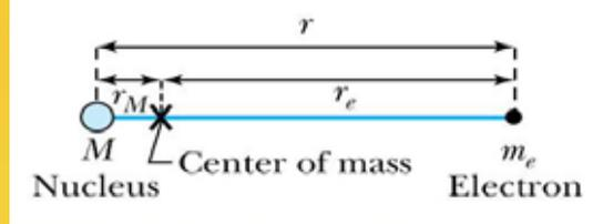
$$\mu_e = \frac{m_e M}{m_e + M} = \frac{m_e}{1 + \frac{m_e}{M}} \quad \text{reduced mass}$$
