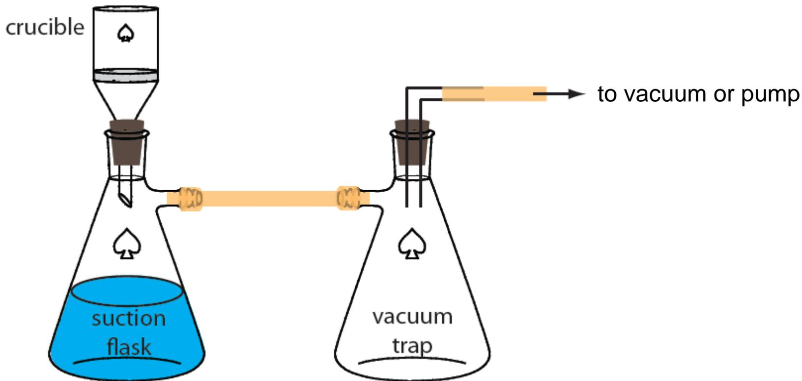
Procedure for filtering a precipitate through a filtering crucible. The trap prevents water from an aspirator from back-washing into the suction flask.
