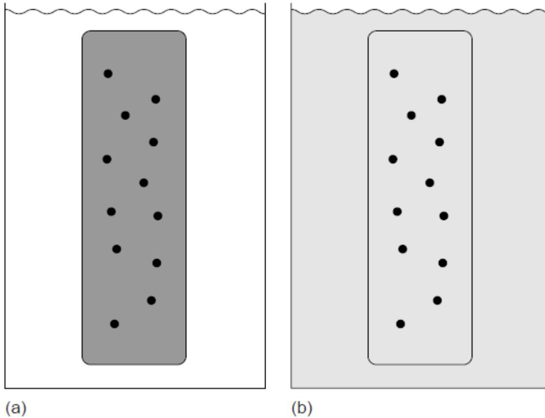
Illustration of a dialysis membrane in action. In (a) the sample solution is placed in the dialysis tube and submerged in the solvent. (b) Smaller particles pass through the membrane, but larger particles remain within the dialysis tube.
