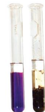
Hexane does not react with purple \text{KMnO}_4 (left); cyclohexene (right) reacts, producing a brown-black precipitate of \text{MnO}_2 .
