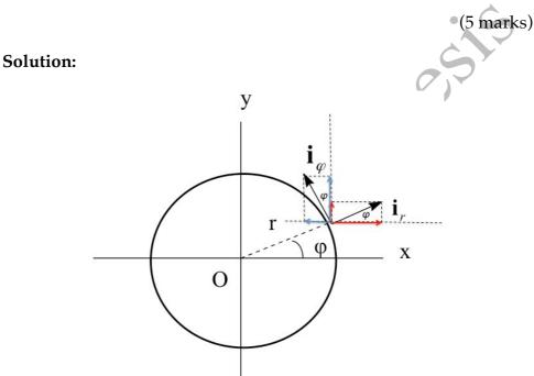
As the figure shows the two vectors  $\mathbf{i}_r$  and  $\mathbf{i}_{\varphi}$  can be resolved into two components along the *x*- and *y*-directions. From the figure we have:
